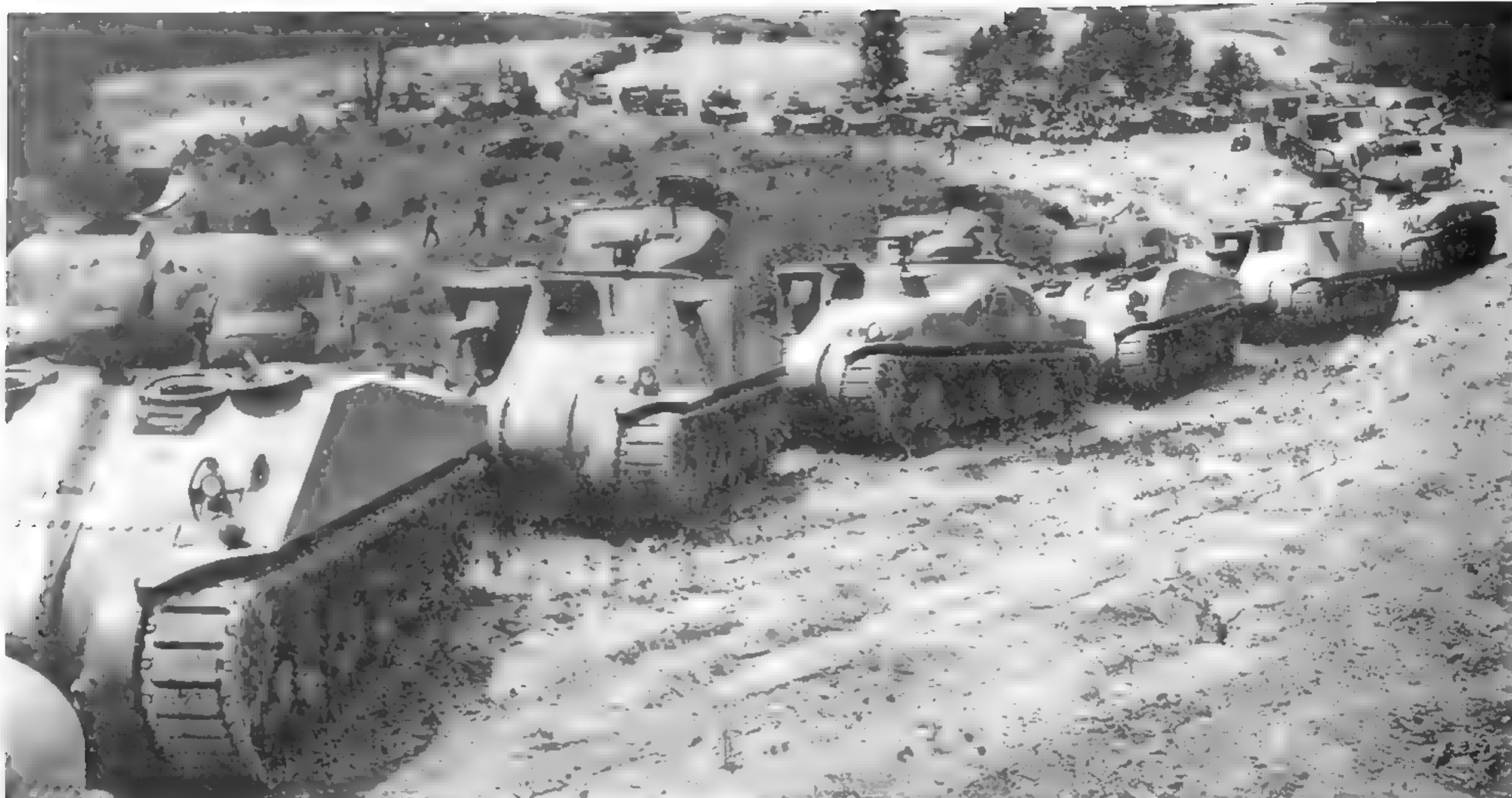
Here are a variety of early WWII medium tanks. In the foreground are an early M4 (note direct vision slots and early VVSS), M3 Lee, M3A1 (notice cast hull), M4A3, M3, M4A1, M3A1, M3, and another M3, followed by eight Stuart light tanks and assorted half-track and wheeled vehicles. (Photo courtesy of the Patton Museum)
